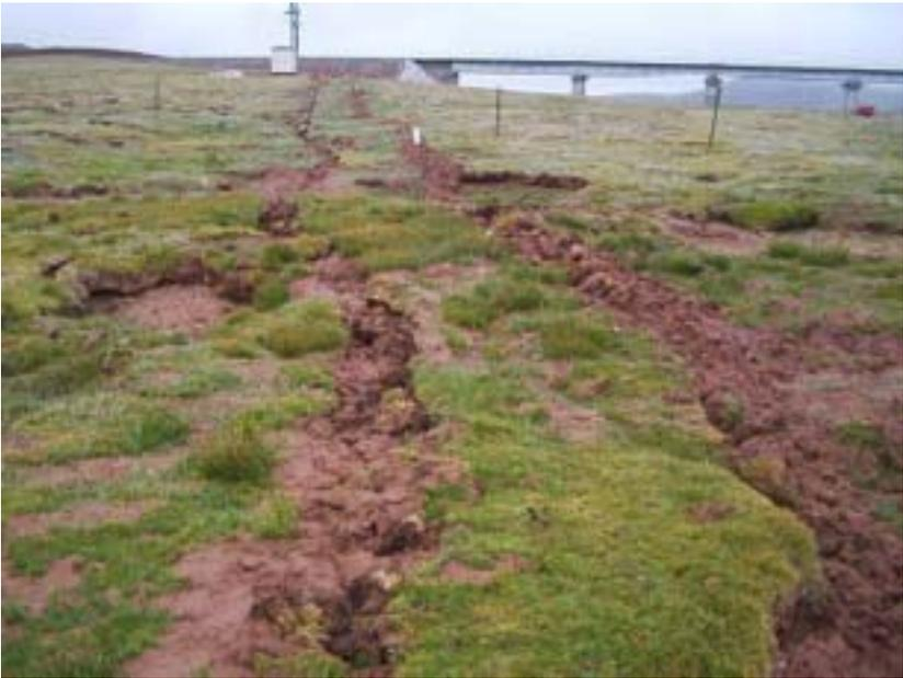
*Surface degradation associated with thaw of ice-rich permafrost on the Tibetan Plateau. As melted ice drains away the soil slumps and collapses*
